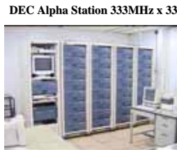
DEC Alpha Station 333MHz x 33 Cisco Catalyst 5000 Fast Ethernet switch 12x3 + 2 port 1.6Gbps Back Plane
