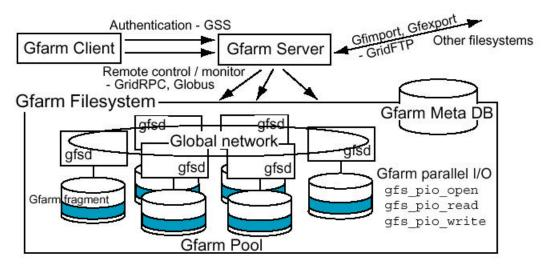
Fig. 1 : Software architecture of the Grid Data Farm
